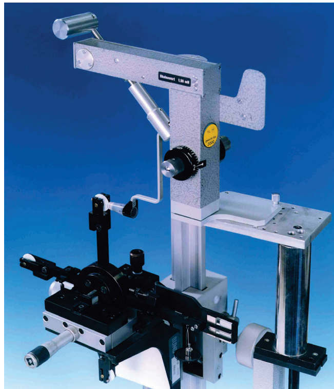
Figure 3 – Detailed view of applanation tonometer test setup (using a balance)
