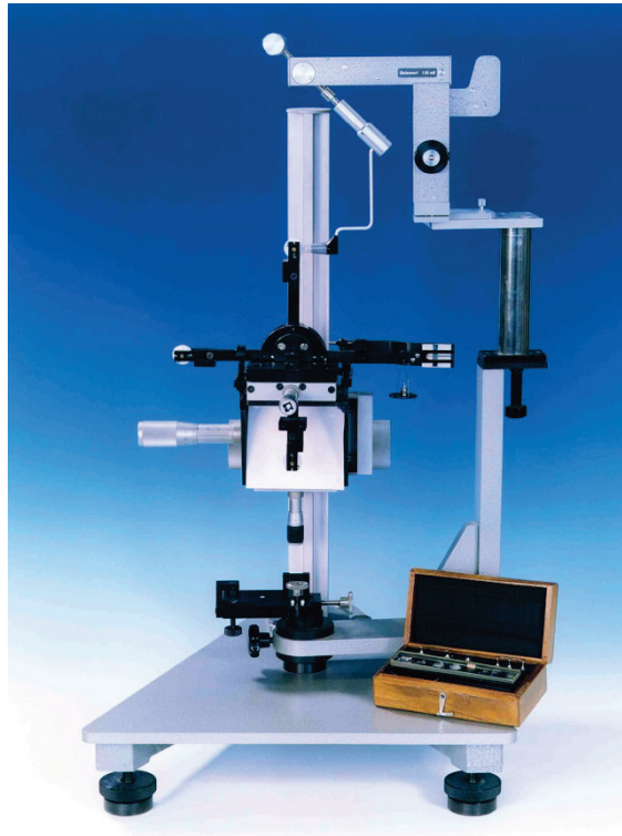
Figure 2 – Applanation tonometer and test setup (using a balance)
